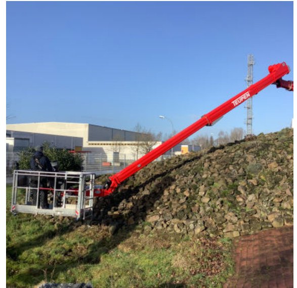
Working in negative areas up to 9,20 m / 13,15 m
