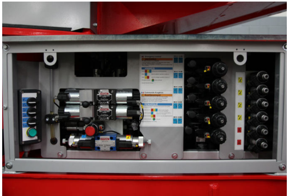
The electric emergency lowering system is easily accessible and follows a self-explanatory 1-2-3 principle
