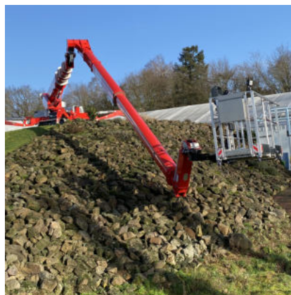
Rotatable platform: 2x 220 ° Movable jib: 200°
